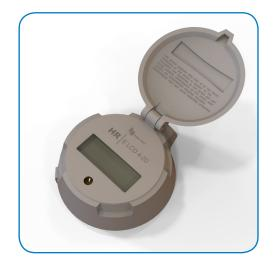
Construction: The housing of the HR-E LCD 4-20 encoder is constructed of an engineered polymer enclosure and a polycarbonate lens. For long-term performance, the enclosure is fully encapsulated, weatherproof, and UV-resistant to withstand harsh environments and to protect the electronics in flooded or submerged pit applications. A patented epoxy potting comprises the encoder bottom. Due to this unique sealing, the HR-E LCD 4-20 exceeds all applicable requirements of AWWA Standard C707.
